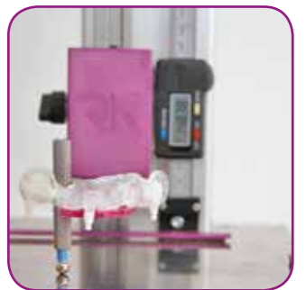
Acquisition of precise measuring values in µm-accuracy for comparison of accurate positions of the permeation opening in the test protocol
